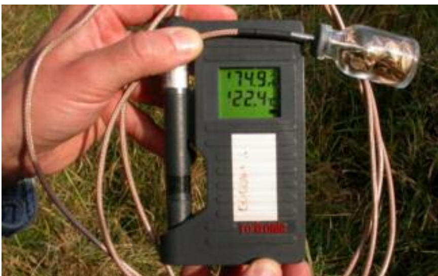
Modified hygrometer allows field measurements of seed moisture content (Robin Probert)
