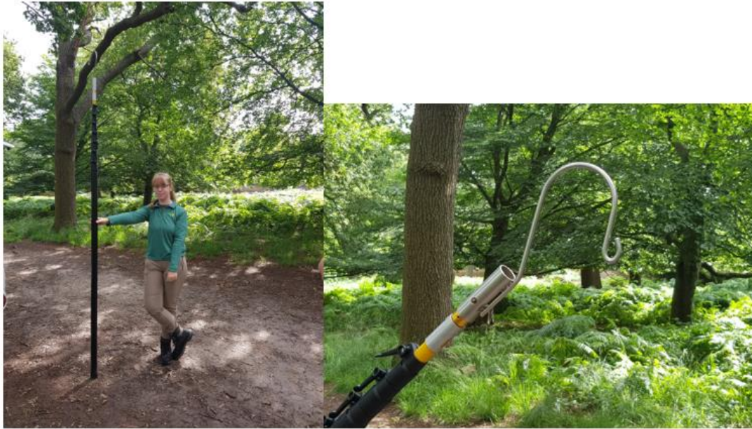
Figure 8. Telescopic extension pole and hook attachment used to place the multi-funnel traps
