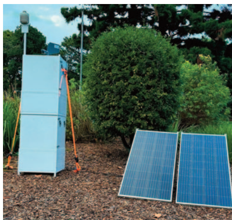
A spore sampler to detect incursions of new strains of myrtle rust at the Royal Botanic Garden Sydney.
